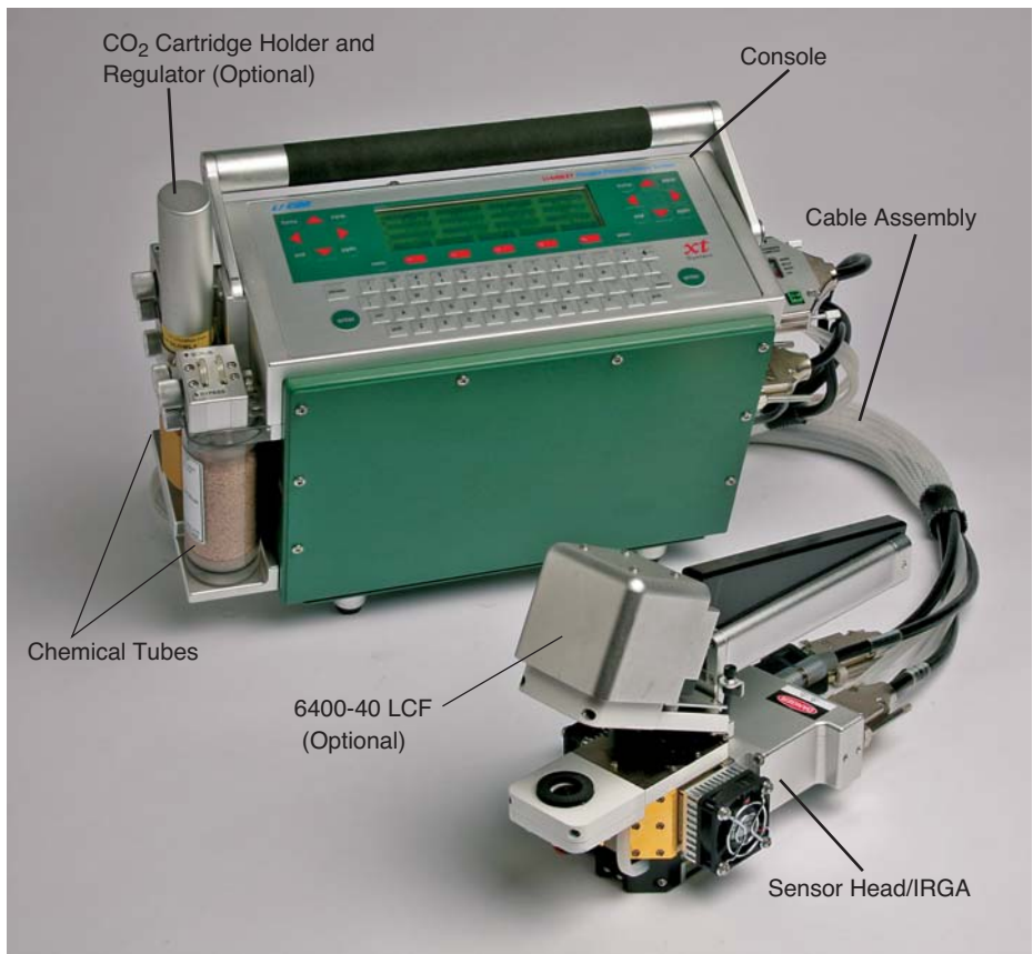
Figure 1-5. The LI-6400XT Portable Photosynthesis System.
