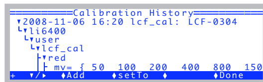
Figure 27-61. Results from Calib Menu|LCF Source|Calibrate will show up in the calibration history (Calib Menu|View Settings|View History).
