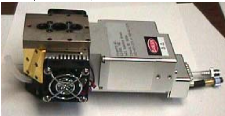
Figure 16-74. The attachment plates mounted on the sensor head.
