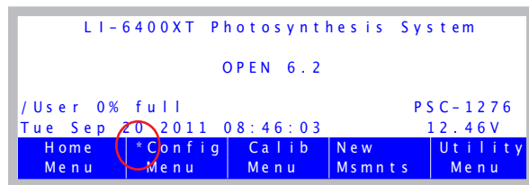
Figure 3-100. The asterisk in the Config Menu label indicates that something has changed.
