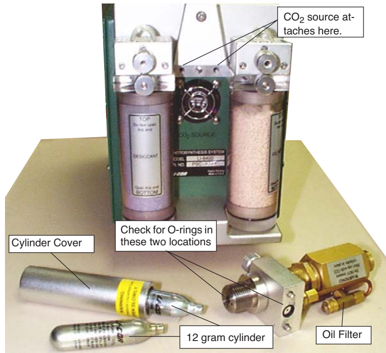
Figure 2-6. Location of external CO 2 source assembly.
