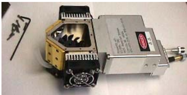
Figure 16-72. The LI-6400 sensor head, leaf chamber removed.
