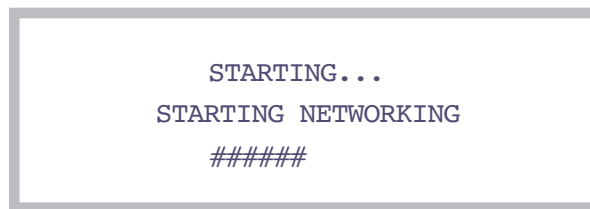
Figure 20-1. The version 6 startup screen. If it is not an XT, the middle line will be blank.
