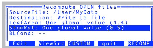
Figure 13-5. Ready to recompute. We'll be setting a new leaf area, and a new stomatal ratio. The recomputed data will be written to an as yet unnamed file.
