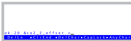
Figure 3-49. Forcing a 20 ppm mismatch in the IRGAs.
