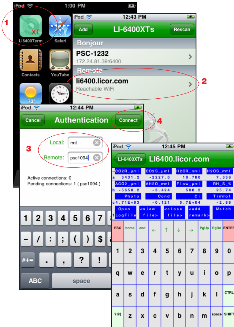
Figure 11-46. Connecting to li6400.licor.com with an iOS device.
