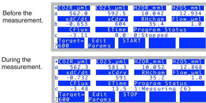
Figure 16-101. Program Status and ETime (elapsed time) indicate the state of a measurement.
