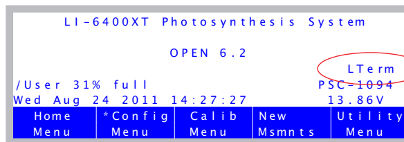
Figure 11-48. LTerm is toggled by pressing L . When active, LTerm allows remote monitoring and control via the RS-232 port.
