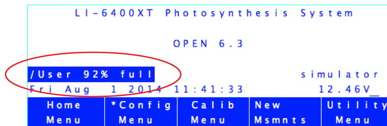
Figure 8: /User disk space is shown in inverse when > 90% full. Above 95%, the message will be blinking as well.
