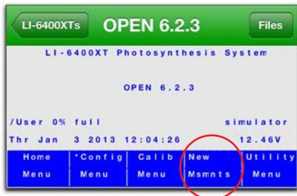
1. Starting at the Main Screen, touch F4 to go to New Measurements.
